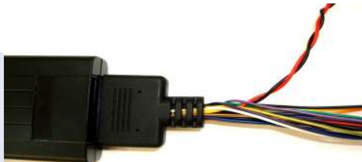
Figure 17 twisting the wires
