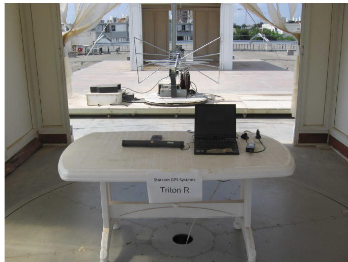
Figure 8. Radiated Emission Test
